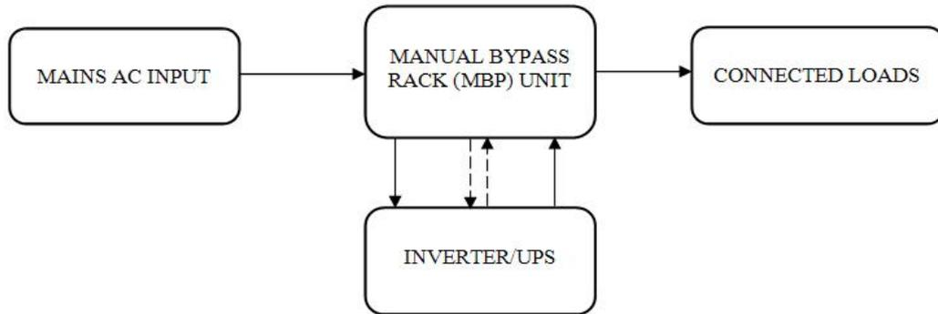
2. Under maintenance operation, the Mains AC Input flows through the MBP unit to the connected Loads – the UPS is not in the circuit.
